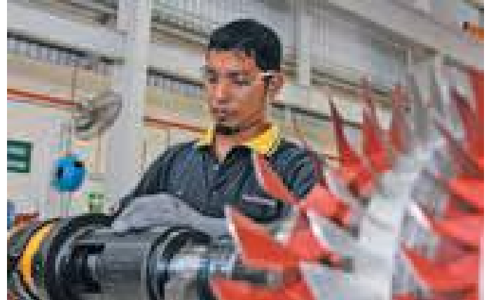
Overhaul of gas turbine
